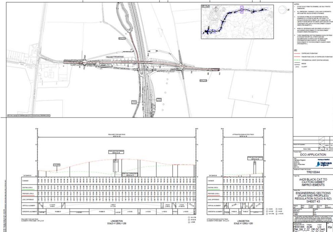
Figure 1: Applicant's General Arrangement and Longitudinal Section of Toseland Road [Extracted from APP-022].
